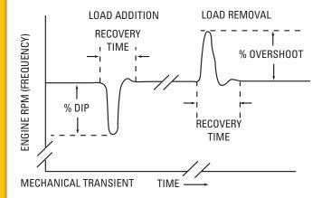
Dips are generally more critical than overshoots because severe block loading can stall the engine and cause generator voltage to collapse. The genset's rotating mass helps maintain frequency, but inertia must be closely balanced between the generator and engine. This is an important factor when specifying an oversized generator, because the frequency dip decreases and allows more engine horsepower to be available for recovery.
