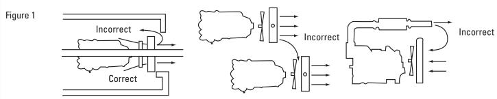
Make sure that radiator installation in enclosures does not cause recirculation of heat or exhaust fumes.
