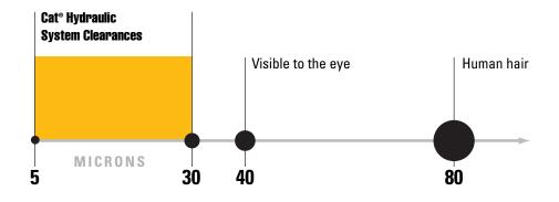
Typical metal-to-metal clearances in Cat® hydraulic systems are 5-30 microns (one micron is one millionth of a meter). Therefore, even particles too small to see can do big damage.
